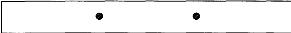
Example 1: Two 1/8 in. (3.2 mm) discontinuities
