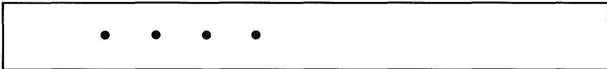
Example 4: Four 1/16 in. (1.6 mm) discontinuities
